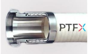
The standard machined internal surface finish of Puresil- Techniflex end fittings is 05µM Ra or better, improved surface finishes can be achieved by Electro Polishing.
